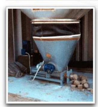
Compacting machine for buffing powder, cheaper than bigger sister "IMPACT D1".
